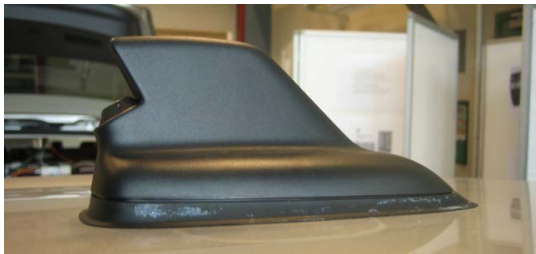
Fig. 1. The conventional antenna housing of a Volkswagen Touran.
