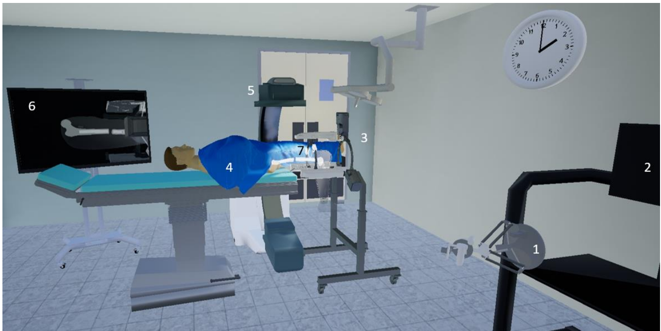
Figure 7. Robossis-assisted femur fracture surgery environment was designed to include (1) a haptic controller, (2) a surgeon workstation, (3) the Robossis surgical robot, (4) a cadaver patient, (5) a C-arm X-ray machine, and (6) real-time visual rendering for the location of the bone is displayed as a 2D fluoroscopic imaging. Robossis surgical robot is attached to the distal bone segment using surgical rods (7). The environment was created with the goal to immerse the trained users in a similar operating room environment for femur fracture surgery using the Robossis system.
