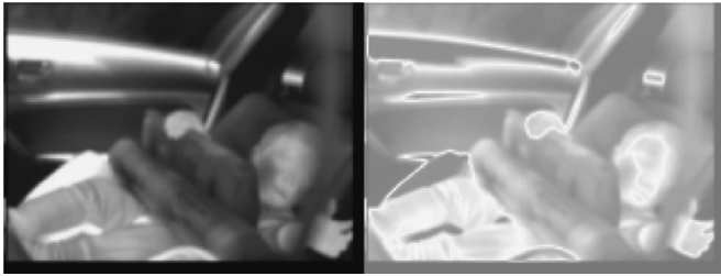
Fig. 15. LWIR images before and after intensity to probability of skin-temperature mapping. Note that areas containing human skin are now bright relative to other objects in the scene.
