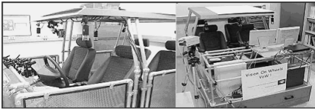
Fig. 4. Laboratory for Intelligent, Safe Automobiles-M (LISA-M) test bed for data collection and algorithm development.
