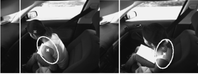
Fig. 12. Examples of unsuccessful head detection due to invalid disparity data because of camera limitations.
