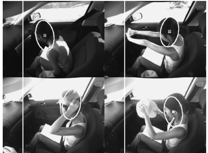
Fig. 11. Examples of successful stereo-based head detection and tracking of an occupant in four different situations.
