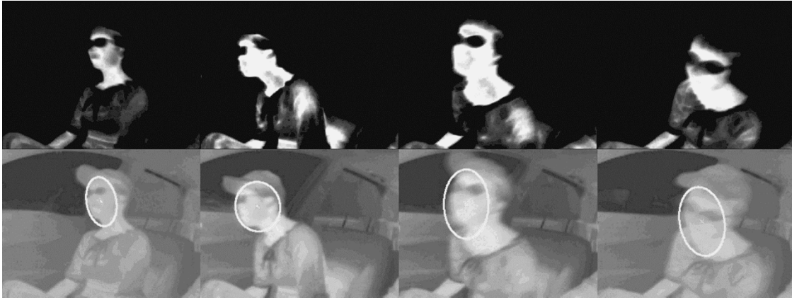
Fig. 16. Inferring head depth from ellipse size estimation in LWIR images.
