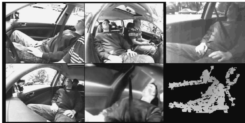
Fig. 7. Example acquired image data from LISA-P. Top left, top middle, bottom left: Multiple perspective NTSC images. Bottom middle: LWIR image. Top right: One of three grayscale images for depth map calculation. Bottom right: Resulting depth image from stereo correspondence.
