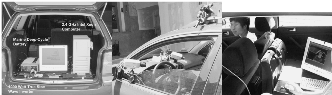
Fig. 6. Top left: LISA-P test bed with the power supply, PC-based capturing system. Right: Three NTSC cameras (front driver and passenger windows and front dash), thermal camera (front dash), and a stereo camera (roof rack) in view. Bottom: Test subject in LISA-P during an experiment.
