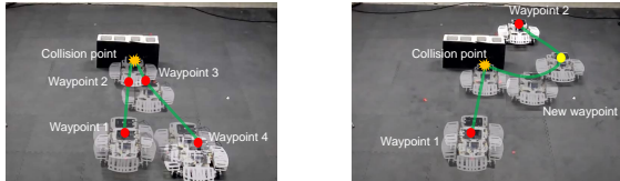
Fig. 8: Composite images (taken every 2 s) of a sample experiment with DRR. The robot must go from start to goal passing through all waypoints, including intermediate ones created post-collision.
