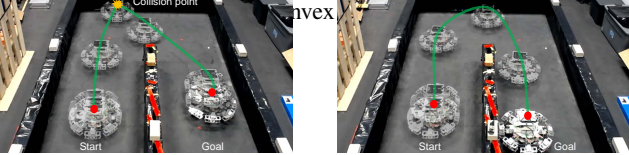
Fig. 15: Composite images of a sample experiment with our unified collision-inclusive motion planning and control framework (left) and of a collision avoidance sample experiment (right). Snapshots shown every 2.5 s. (See supplementary video file for more details.)
