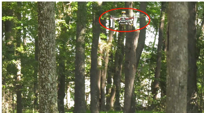
Fig. 16. Single UAV autonomous exploration at NASA LaRC. The vehicle (highlighted in red) performs landmark-based SLAM based on detected trees in order to estimate its position within the forest.
