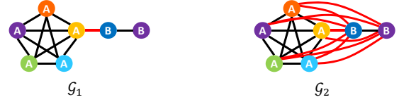
Fig. 7. Evaluating the performance of cycle-inconsistent solutions (e.g., \mathcal{G}_1 ) for clique-centric applications must be done after completing the connected components of the association graphs (i.e., for the transitive closure \mathcal{G}_2 ). Even a single incorrect edge (drawn in red) may have catastrophic consequences in clique-centric applications.
