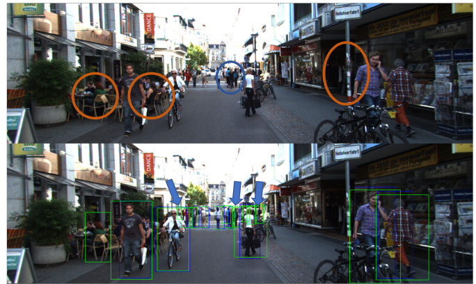
Fig. 13. Visualisations of detection generated by PA-RCNN on KITTI val split for an example image with occlusions and overlaps. Top: the origin image. Bottom: image with the annotations of ground truth bounding boxes in blue and predicted bounding boxes in green. Arrows indicate the correctly detected targets, which are not labelled in the dataset. Orange circles highlight the ambiguous targets associated with the wrong detection shown in Figure 14. The blue circle indicates the target, whose front-facing direction is incorrectly predicted with a Mirror ( xz -plane) transformation shown in Figure 12b.
