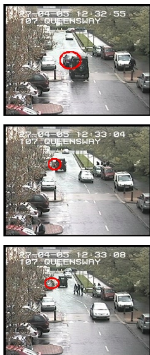
Figure 21. Sequence of images showing a missed detection in sequence PVTEN201b. The occlusion by the SUV car and the tree leaves make this sequence extremely difficult.
