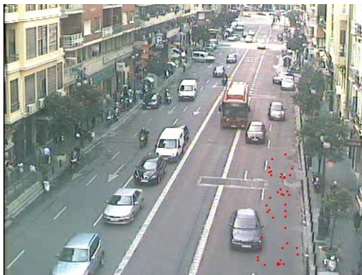
Figure 6. Locations (in red) where static corners will be discarded based on the accumulator of the day before. Notice that some points are located on road markings or dirt. Points on smooth areas are due to cars that were parked at those locations the day before for a long enough time.
