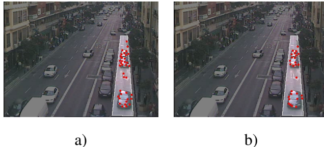
Figure 4. a) Corners detected using Harris detector. b) Corners detected using Tomasi-Kanade features detector.
