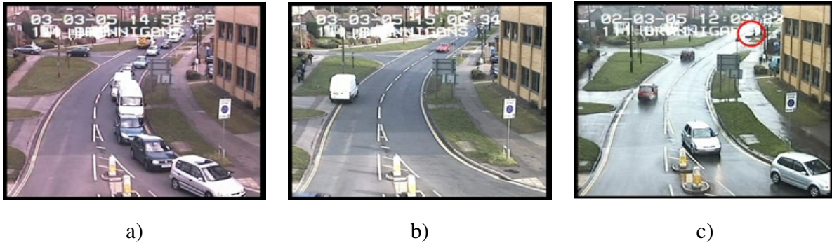
Figure 22. a) Queue that caused a false alarm in PVTEA301c. b) Van that was not detected in sequence PVTEA301c because it was mostly outside of the lane mask. c) Vehicle not detected in sequence PVTEN301c because the overlaid text area was excluded from the detection mask.
