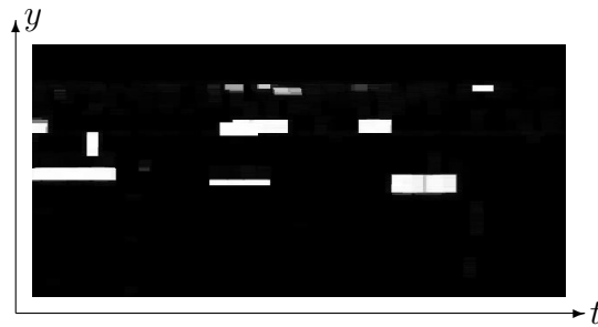
Figure 9. Example of static spatio-temporal map after spatial (vertical) filtering and temporal (horizontal) filtering.
