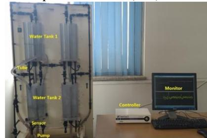
Fig. 7. The water tank experiment setup
