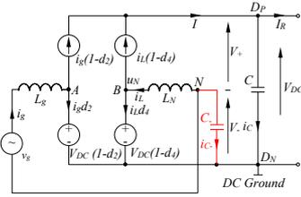
Fig. 3. Average circuit model of the proposed converter.
