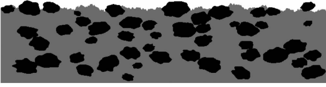
Fig. 3. Soil representation simulated by the soil-geometry simulator. The fine earth is in gray, and clods are in black.
