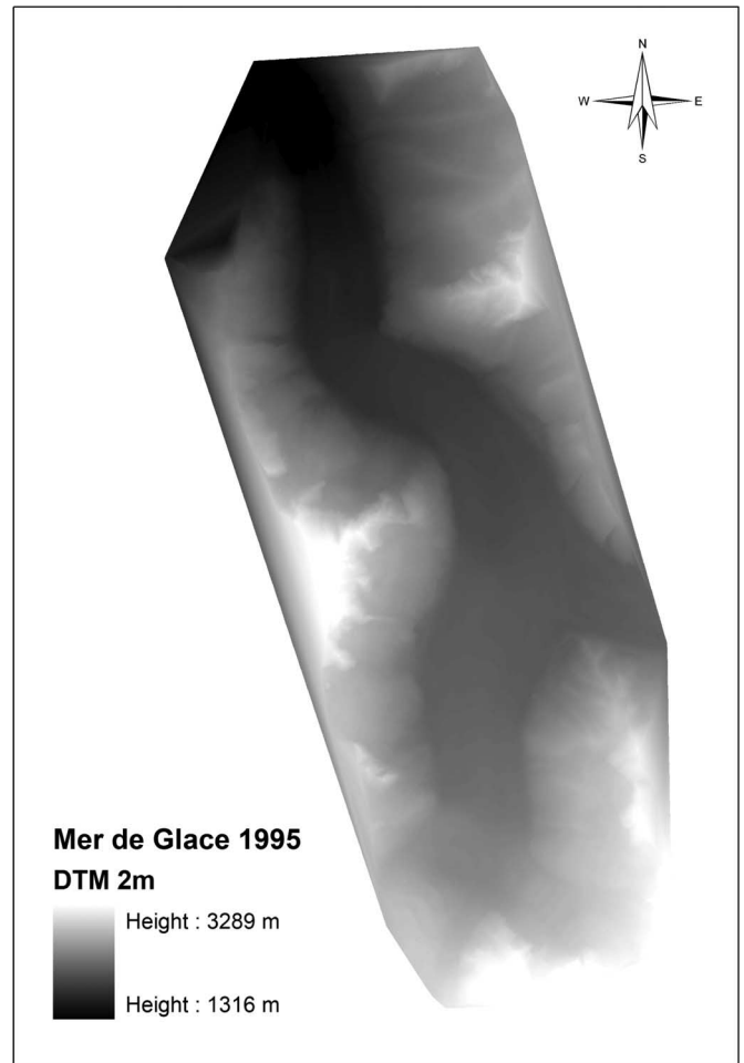
Fig. 4. Mer de Glace DTM processed by photogrammetric techniques.
