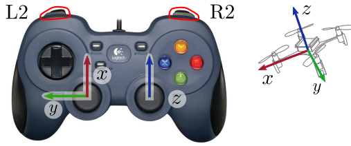
Fig. 10. Joypad used in conditions JN and JV. The left-hand thumbstick commands velocity along the x and y axes of the robot, while the right-hand thumbstick modifies its altitude. The two lower shoulder buttons R2 and L2 increases and decreases the external input \mu_\lambda(t) for the asymptote value of \lambda_2 , respectively.
