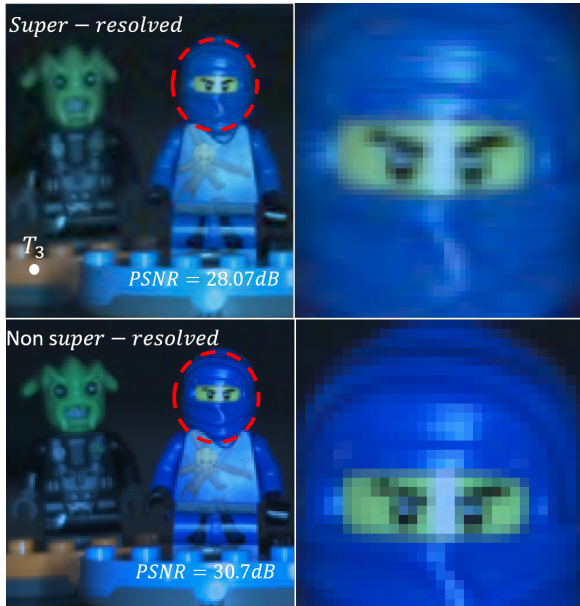
Fig. 15. Top left: RGB profile of the super-resolved 233 \times 256 \times 24 datacube, with s \approx 0.1 , \Delta_c = \Delta_d/2 , and CR = 0.68 . Top right: Zoomed portion of the datacube. Bottom left: RGB profile of the non super-resolved datacube, with s \approx 0.1 and \Delta_c = \Delta_d . Bottom right: Zoomed portion of the datacube indicated by the dashed red circles.
