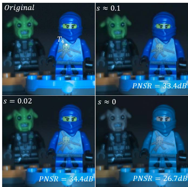
Fig. 18. Original and reconstructed RGB profiles for 3 different coded aperture positions, Q = 6 snapshots and \Delta_c = \Delta_d . The codes exhibit boolean structure. The optimal PSNR occurs at s = 0.02 , while at s \approx 0 the SSCSI does not recover spectral information.
