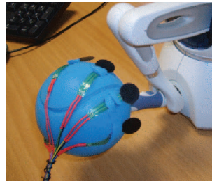
Figure 4: Foam ball with sensors
