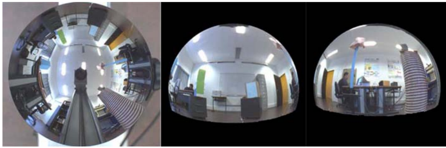
Fig. 9. An omnidirectional image and two views of its projection onto the unit sphere.
