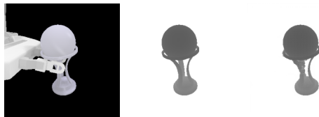
Fig. 7: Left: RGB component of the RGB-D input to the network. Middle: ground truth depth image. Right: Output of Pix2Pix which segmented out the gripper and hallucinated the gaps behind the fingers.
