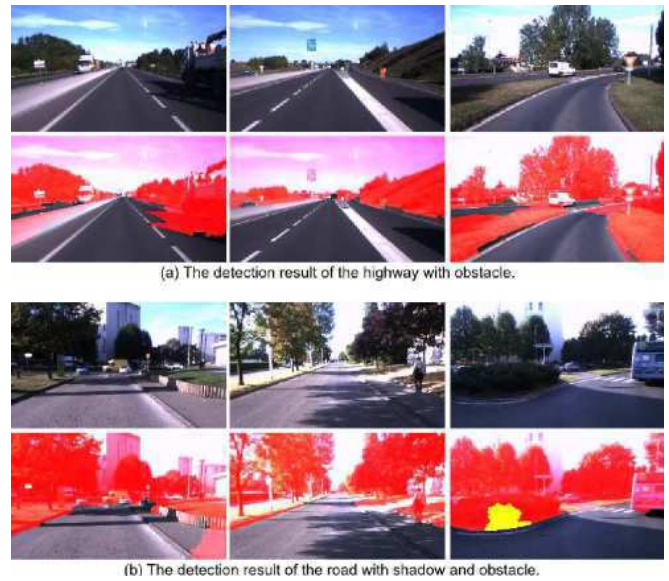
Fig. 8. The original image on top and the classification results on bottom for several conditions, where original colour represents the road detected, the red pixels are the non-road surfaces, and the yellow ones representing the unknown areas.
