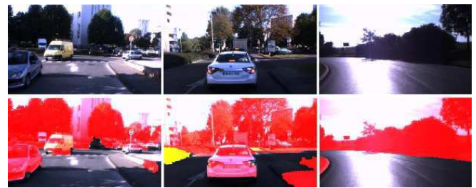
Fig. 9. The original image on top and the classification results on bottom for extreme conditions, where original colour represents the road detected, the red pixels are the non-road surfaces, and the yellow ones representing the unknown areas.
