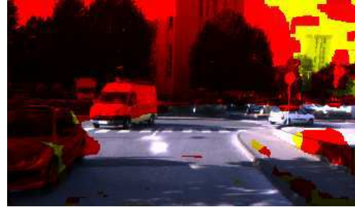
Fig. 7. Final mapping of the free space (original colours), obstacles (red pixels), and elements without any classification (yellow pixels).
