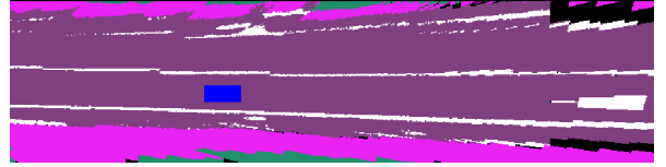
Fig. 5. The semantic map generated by back-projecting 2D semantic image into the 3D space with planar assumption. The map presented in the vehicle frame. The distortion of lines indicates the failure case.
