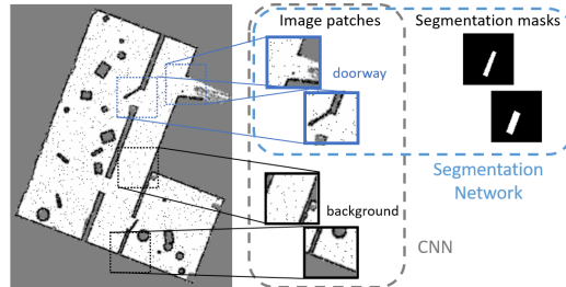
Fig. 6. Generation of training data with our simulator. An occupancy grid map is generated, image patches of certain size are automatically extracted and labeled for training the CNN, and segmentation masks are additionally created for all doorway patches to train the segmentation network.
