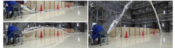
Figure 15. Injecting helium gas into the arm. Helium gas is injected from an inlet port on the base balloon to all balloons through narrow ports between the balloons. 23 min were required from starting (A) to full injection (C).
