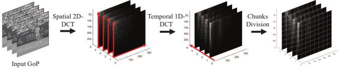
Fig. 2: Compression Step in *SoftCast* scheme. From left to right: GoP in pixel domain, 2D-transformed frames, 3D-transformed frames, Chunks division after 3D-DCT.
