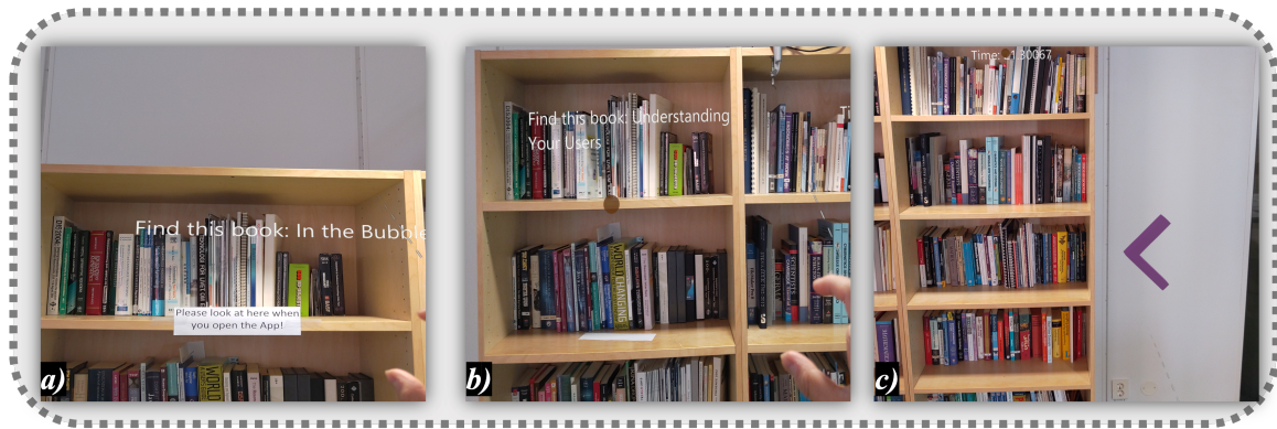
Figure 1: Case study: Visual book-searching task with the aid of AR using HMD. a) : Our AR app gives a book title as a search stimulus. b) : Instant post-task feedback is provided by a dot smoothly following the eye trajectory. (Note: the dot is bright and highly visible in AR but is dim and difficult to see in print; here, it is located between the first and second shelves of the bookcase). c) : The visual hint, as a bright purple arrow, supports the task. The timer is designed for measuring the task time (at the top of this figure). Both the gaze playback and visual hints are rendered in real world space for precise displacement. Please check our supplementary video for the demonstration of the book-searching task.
