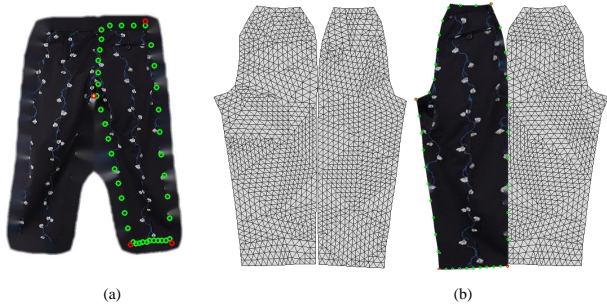
Figure 8: Texture Extraction for Pants. (a) The extrapolated pants image with control points. (b) The image segment is deformed to the desired location on the 2D reference mesh.
