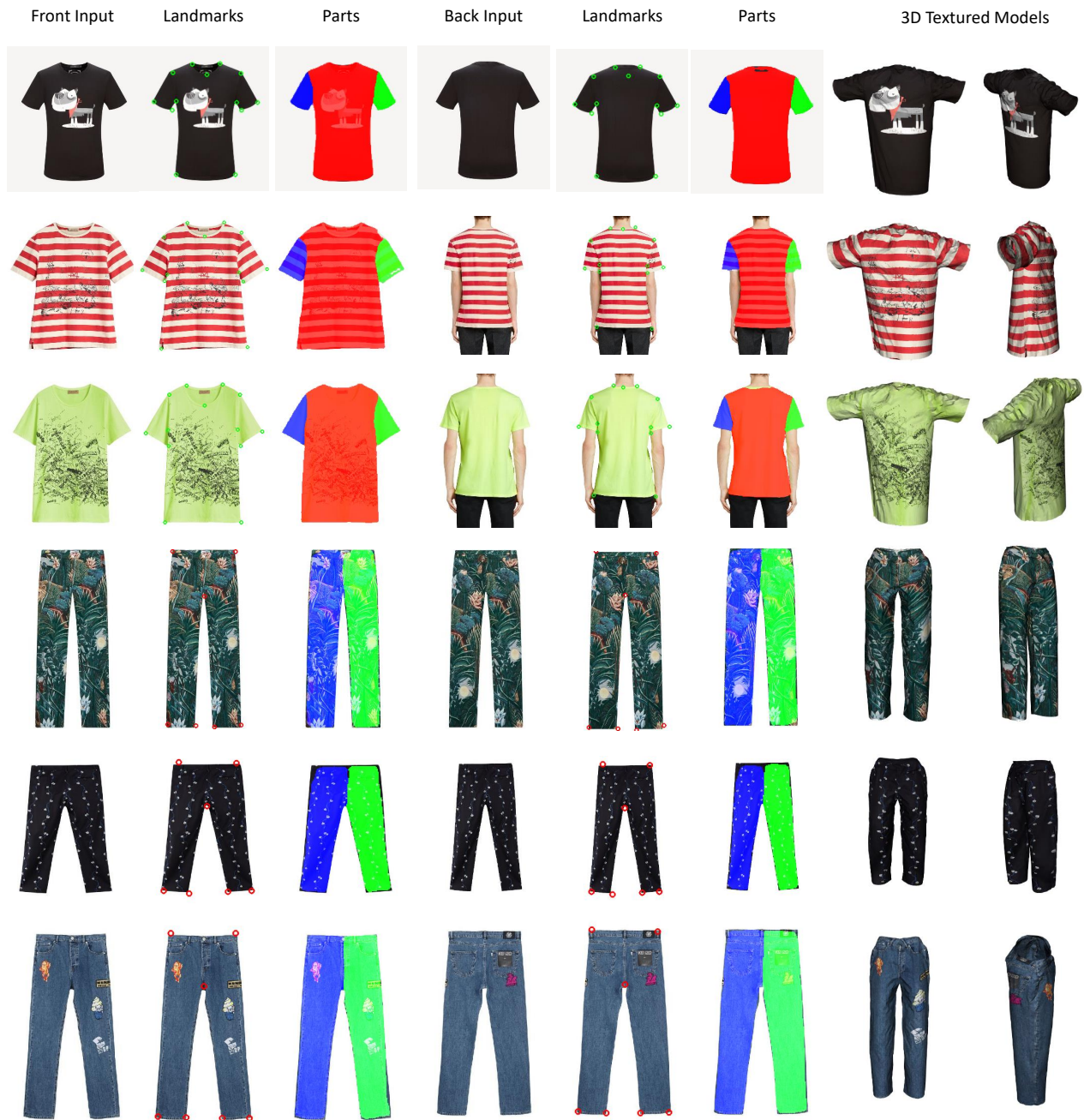
Figure 9: 3D Modeling Results. On each row we show front image and its landmark prediction and part segmentation, followed by back image and its landmark and part segmentation results. The final two columns show 3D textured models for two view points.
