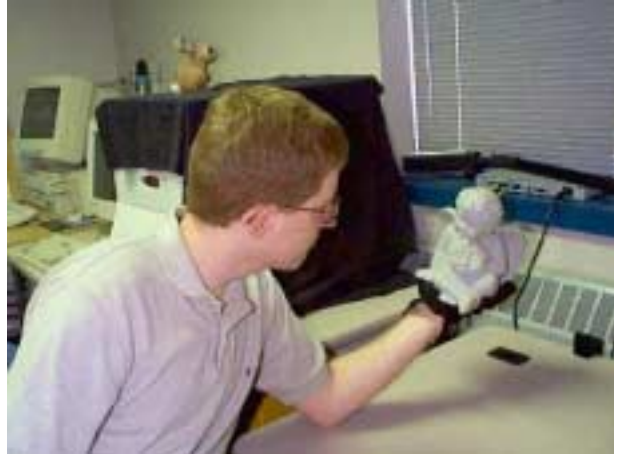
Figure 5: The hand-held modeling application – a 3D model is automatically constructed from scans of an object held in the user’s hand.
