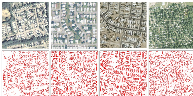
Fig. 1. Line based representation of aerial scenes. We compute local line pattern statistics based on difference in line orientations, length, position within a local neighborhood and line contrast statistics from the image patches to generate higher-order scene features that can yield accurate semantic categorization of the scene. The image patches shown here represent mobile home parks .
