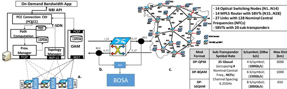
Figure 1. a. T-SDN Controller – OAM Handler Integration; b. Distributed Monitoring System; c. Flexi-Grid Network Topology (detailing link distances in km) and SBVT Capabilities
