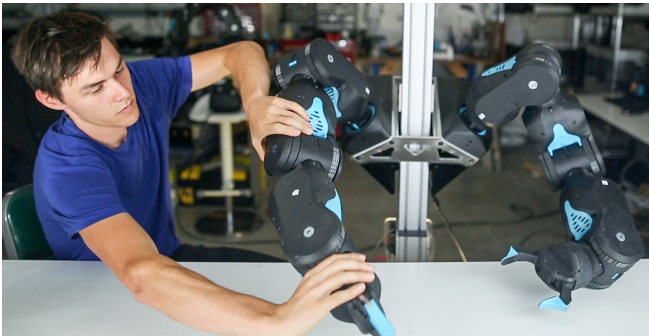
Fig. 4. The Blue arm is designed to minimize pinch points. Safety as a constraint during design heavily impacts the final form of a robot that will interact with human environments. [video on website]
