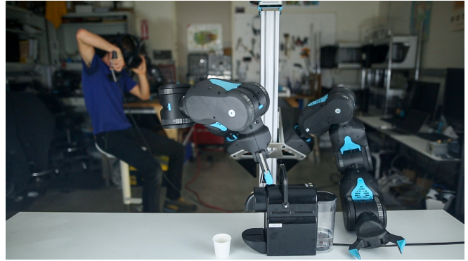
Fig. 5. Blue completely teleoperates an espresso machine. A Virtual Reality operator (in background) pilots Blue using an HTC Vive system through a Unity bridge. A predictable 7-DoF ‘elbows out’ configuration is interpreted from 6-DoF Vive controller pose. Visual feedback is provided by an Intel RealSense D415 depth camera. [video on website]
