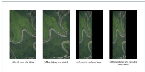
Fig 3 Images to be stitched and distortion processing after projective transformation
