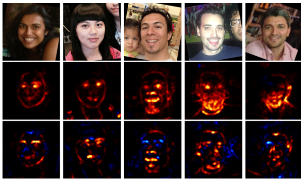
Figure 4. Heatmaps for GoogleNet models and gender recognition. Input images are shown above heatmaps for a DNN pre-trained on Imagenet, which are shown above heatmaps for a DNN initialized randomly. The finetuned model predicts based on an ensemble of facial features, whereas the model starting with random weights has overfit on an isolated set of features characteristic to the target classes.
