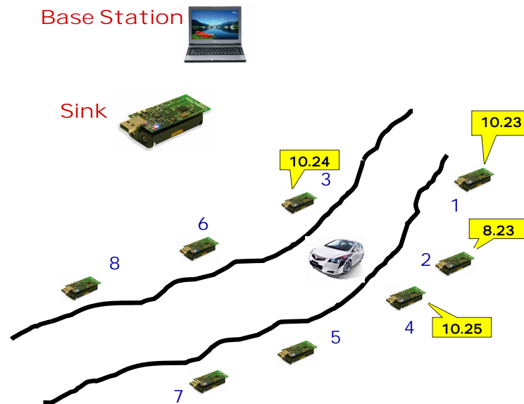
Figure 4: Motes sense the motion of the car and record their local time at the time of event.
