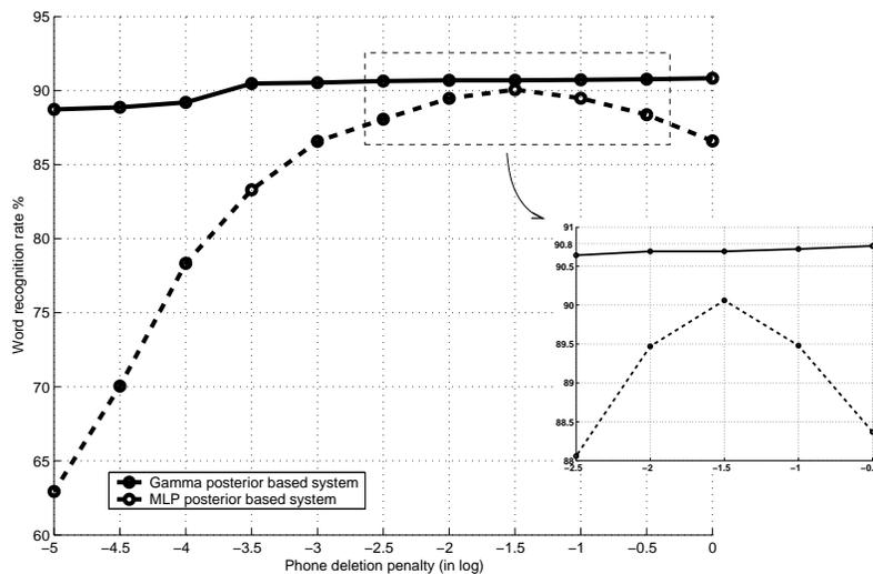
**Fig. 2.** Comparing the sensitivity of gamma posterior based system and MLP posterior based system to tuning phone deletion penalty. The diagram inside is a zoom of performance curves for small values of phone deletion penalty (fine tuning).
