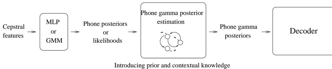
**Fig. 1.** The whole recognition system. First, initial phone evidences are estimated using GMMs or MLPs, then these evidences are used to estimate gamma state posteriors through a HMM, which are then integrated into phone gammas. Finally, phone gammas are used as local scores for decoding.
