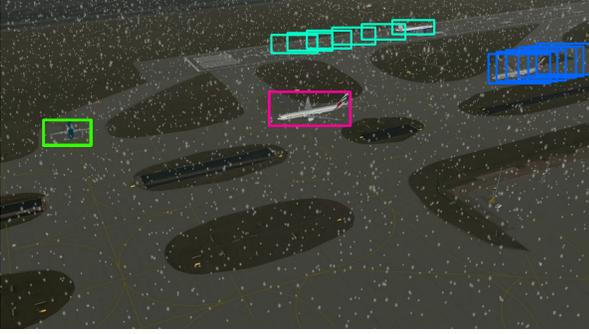
Figure 6: Aircraft tracking by detection. By comparing aircraft bounding boxes from previous frames, the algorithm can map them with the current frame.
