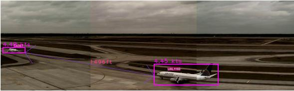
Figure 15: Aircraft detection and speed/distance estimation by Deep4Air framework.
