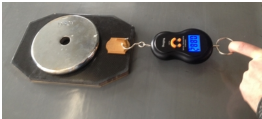
Fig. 3. We estimate the coefficient of friction of a material by several measurements of the maximum friction force on the robot foot, loaded with a 1.5kg mass.
