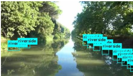
Fig. 8: Detections generated by Tiny-YOLO v3 on a particular image with a complicate environment (shadow of trees).
