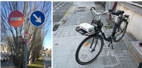
Fig. 10. UWB anchor and bicycle positioning prototype.
