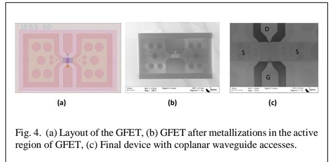
Fig. 4. (a) Layout of the GFET, (b) GFET after metallizations in the active region of GFET, (c) Final device with coplanar waveguide accesses.
