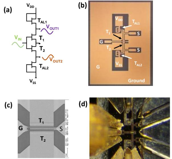
Fig. 6. Balun circuit: (a) Electrical circuit of the GFET balun, (b) Optical image of the balun circuit fabricated, (c) SEM image of  $T_1$  and  $T_2$  configuration highlighting the layout; (d) Photography of the balun circuit under measurement condition. Chip size is 0.19mm<sup>2</sup>.
