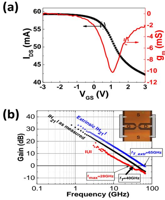
Fig. 5. Performance of GFET on SiC: (a) DC characteristics of bilayer graphene on SiC with  $L_g = 150$  nm,  $W = 2 \times 15$   $\mu$ m. The evolution of the drain current  $I_D$  and the transconductance  $g_m$  as a function of the gate voltage  $V_{GS}$  at  $V_{DS} = +1.5$  V, (b) RF gain performance measured on the probe plan (as measured) and the de-embedded values from which cut-off frequencies are deduced ( $f_T$ ,  $f_{max}$  and extrinsic value  $f_{T\_extr}$ ).
