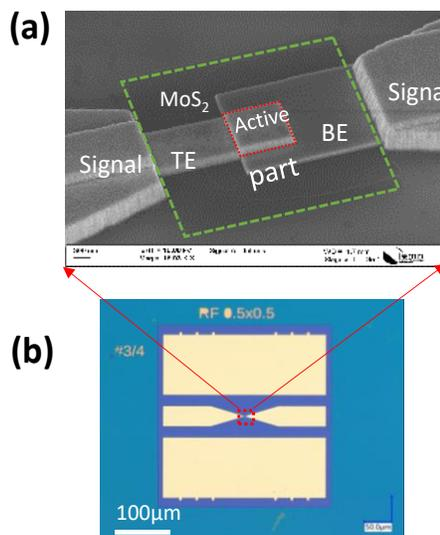
Fig. 8. (a) SEM image of the vertical resistive switch with gold as bottom electrode (BE),  $\text{MoS}_2$  as dielectric and gold as top electrode (TE). The active size is  $0,5\mu\text{m} \times 0,5\mu\text{m}$ ; (b) Resistive switch embedded in a coplanar waveguide for RF applications.
