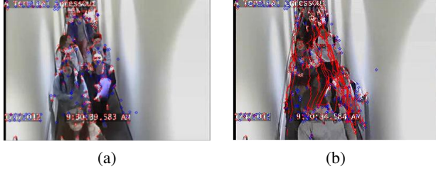
Figure 8. Results of feature tracking. (a) Features detected in the image. (b) Point tracks extracted from a video sequence.
