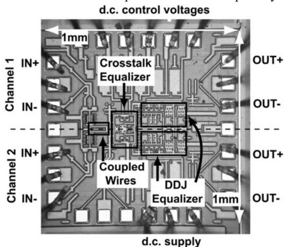
Fig. 4. Chip microphotograph of the XTC and DDJ equalizers.
