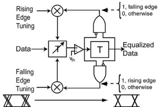
Fig. 3. Schematic for DDJ equalizer with independent rising and falling edge jitter.
