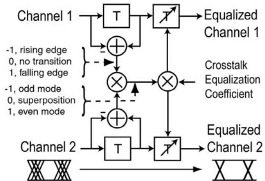
Fig. 2. Schematic of a two-channel crosstalk-induced jitter cancellation.
