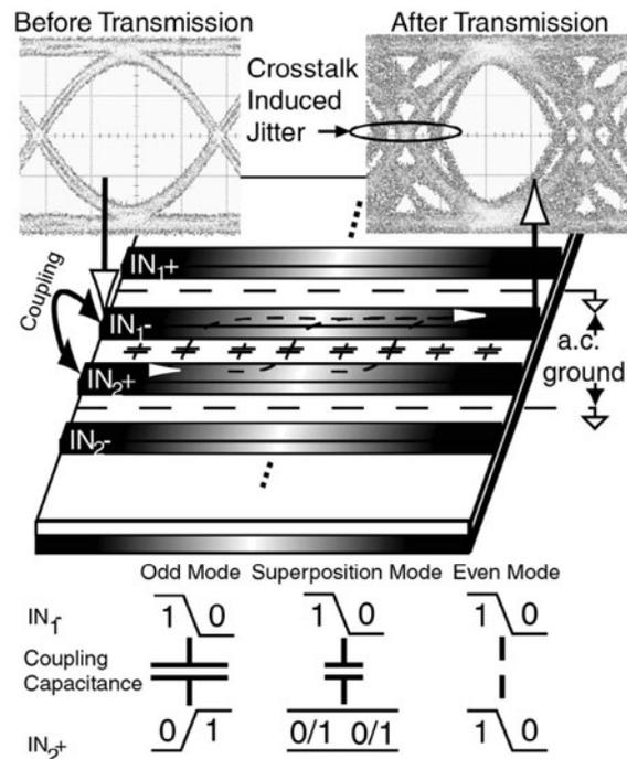
Fig. 1. The crosstalk jitter generated in the data eye due to the influence of a neighboring signal. Three possible modes can occur between transitions on neighboring lines.
