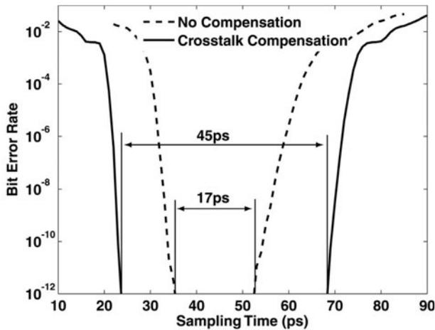
Fig. 6. Bathtub curve resulting before and after equalization.
