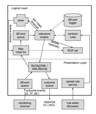
Fig. 6. Architecture of the Contract Compliance Checker (CCC).
