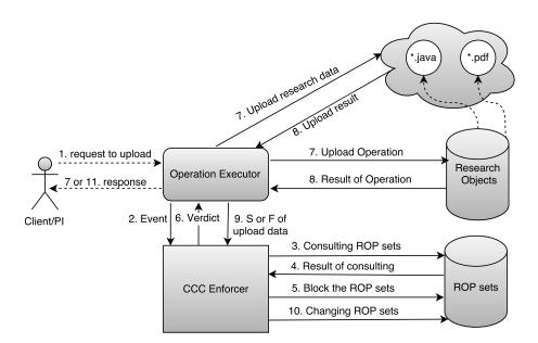
Fig. 3. Typical interaction with the CCC Enforcer.
