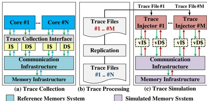
Fig. 1. Structural view of trace-driven simulation phases.
