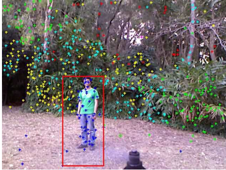
Fig. 5. 2D projections of clustered 3D points on the image plane. Color is associated with corresponding 3D cluster. Bounding box in red is estimated based on projected points. (This figure is best viewed in color).
