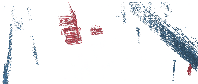
Figure 8. Motion segmentation. The red points have larger motions relative to the blue points. A truck, car, and pedestrian (bottom right) were segmented from the Argoverse Scene Flow scene.
