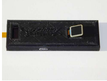
Fig. 6. The tested Multi-Biometric Authentication Device (MBAD) prototype
