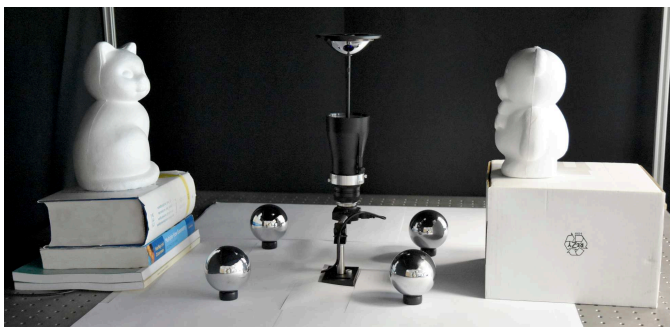
Fig. 12. Real-world experiments: catadioptric camera, Cat and Teddy Bear , and the four mirror balls used for the estimation of the illumination vectors.
