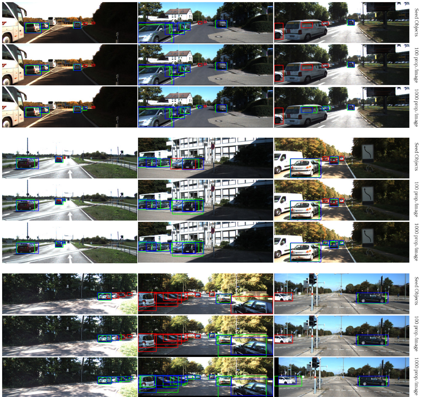
Figure 5: Object proposals generated in chronological order using the context-based strategy based on camera-centered higher-order relations. Matched object annotations are marked in blue, missed detections are marked in red and matching object proposals are color-coded in green. First row, seed objects collected with the object detector [18]; second row, results after sampling 100 object proposals; and third row, results after sampling 1000 object proposals (Best viewed in color).
