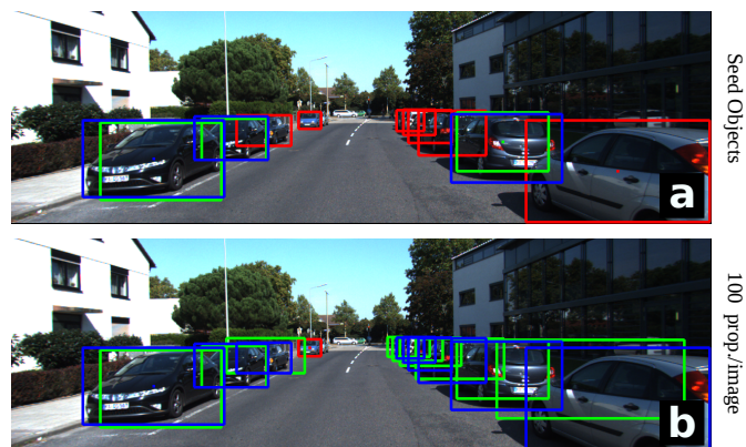
Figure 1: Object detections collected: a) after running a standard appearance-based detector, b) after sampling 100 context-based object proposals post detection. Notice how we manage to recover many of the initially missed detections. Matched annotations are marked in blue, missed detections in red and matching object proposals in green (Best viewed in color).
