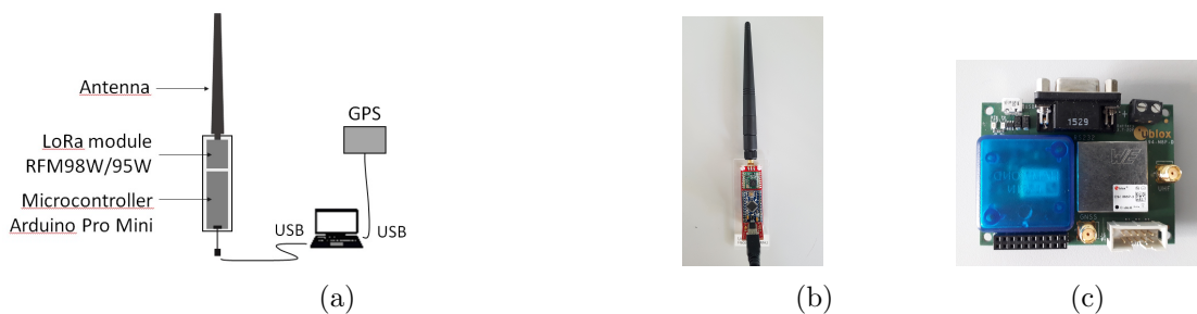
Figure 4: Receiver node RX: a) Principle scheme, b) Node, c) GPS (u-blox C94-m8p)
