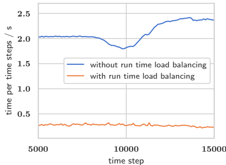
Figure 9: Hopper discharge simulation on the JUWELS supercomputer using 1296 cores. The computation time per time step without load balancing (blue) is considerably higher than for a simulation with run time load balancing enabled (orange).
