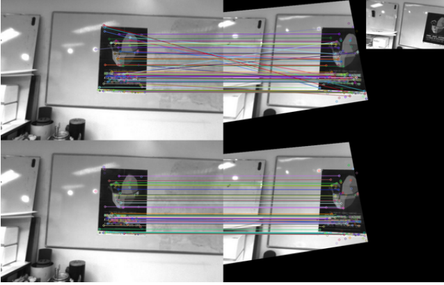
Fig. 2. Matching point correspondences between the warped image frame 264 (warped by the predicted homography) and the reference frame. Poor matching (top) and excellent matching (bottom) before and after applying our outlier removal procedure. Reference frame (left), warped current frame (right), current frame (small image on top right corner).
