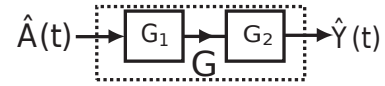
Fig. 1. The cascade connection of two linear quantum systems: G = G_2 \triangleleft G_1 .
