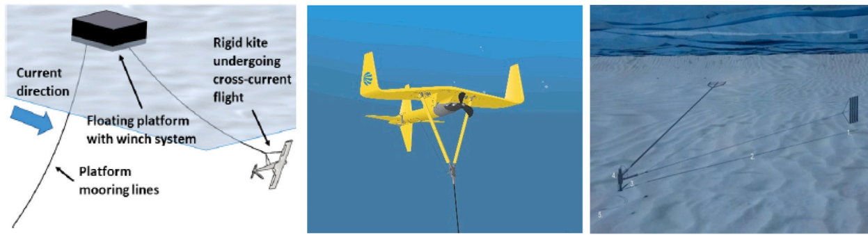
Fig. 30. Major components of an ocean kite system (Cobb et al., 2019a); Minesto Deep Green (Minesto, Ltd, 2021); and SeaCurrent Tidal Kite (SeaCurrent Holding BV, 2021).
