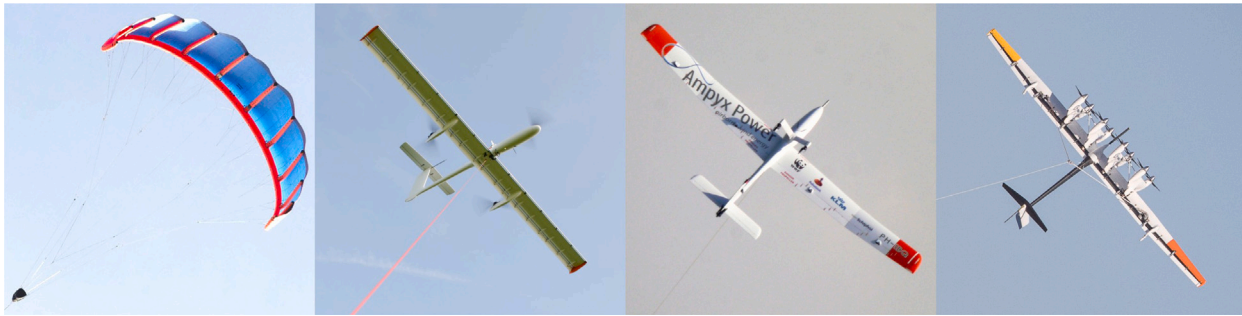
Fig. 1. Selected AWE systems currently in development: Kitepower, TwingTec, Ampyx Power and Makani Power (from left to right), generating up to 600 kW per single system . Source: Photos from Schmehl and Tulloch (2019).
