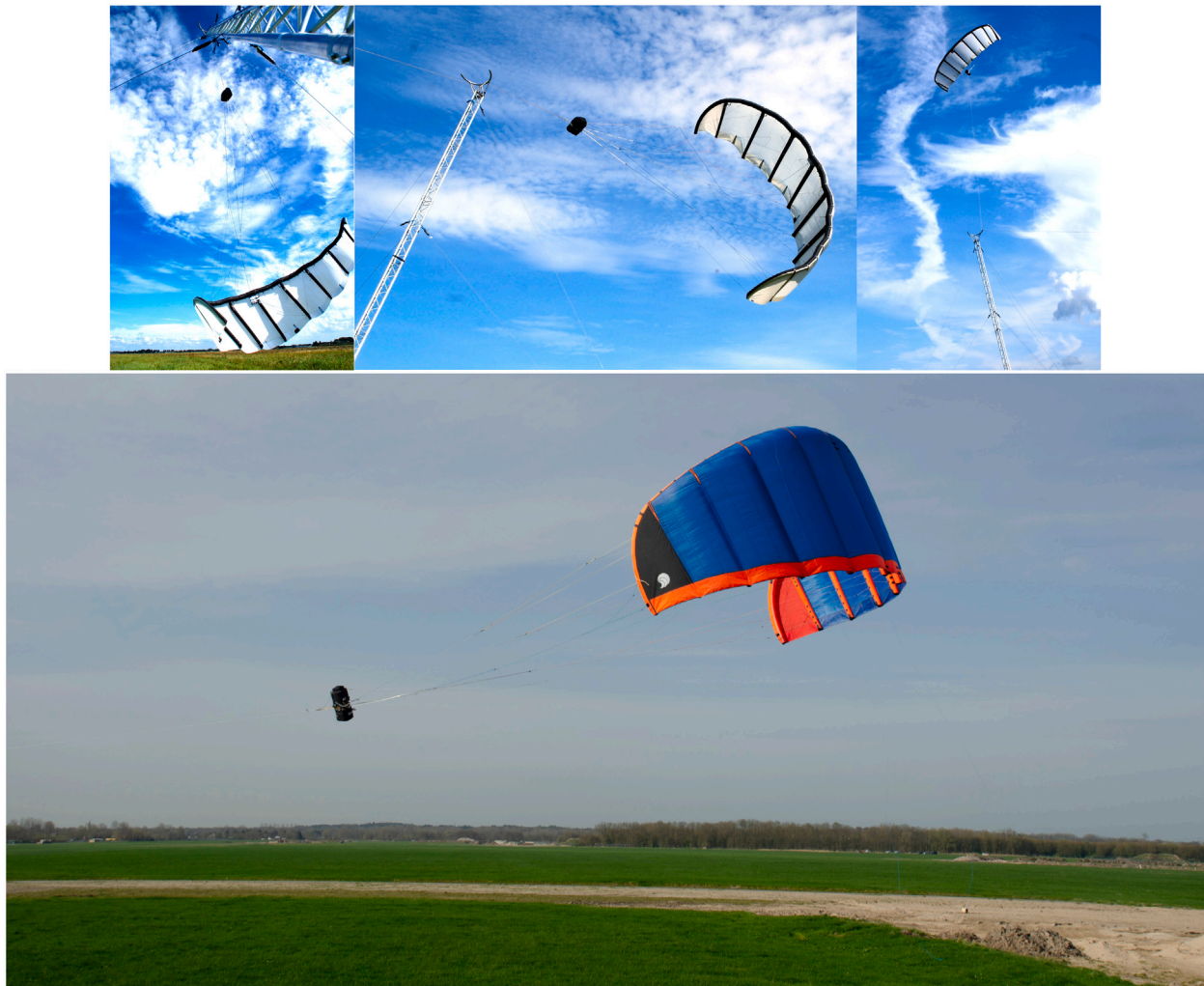
Fig. 26. Experimental launch of a 25 m 2 V3 leading edge inflatable tube kite from an upside-down hanging position on 23 August 2012 (top), standard half-automated winch launch of a 40 m 2 V5.40 derivate kite, temporarily reaching a tether force of 15 kN and a mechanical power of 100 kW during a test flight in May 2018 (bottom) (Kitepower, 2018).
