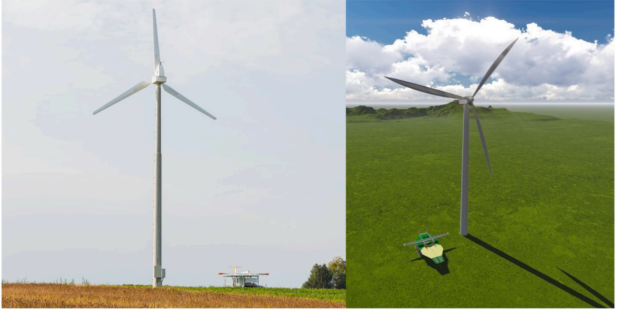
Fig. 3. Conventional wind turbines next to docked AWE systems of comparable rated power: photo of the TwingTec pilot system (Luchsinger et al., 2019) (left) and rendering of the envisioned offshore system of Ampyx Power, the AP4, with a rated power of 2 MW (Kruiff & Ruiterkamp, 2018) (right).
