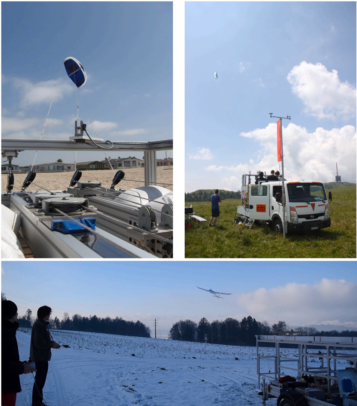
Fig. 29. Examples of prototypes for field tests whose results and data are available to the research and development community. Clockwise from top left: UCSB prototype (Fagiano & Marks, 2015; Fagiano et al., 2014), Swiss Kite Power prototype (Zraggen et al., 2016), ABB Corp. Res. prototype (Fagiano et al., 2017, 2018).
